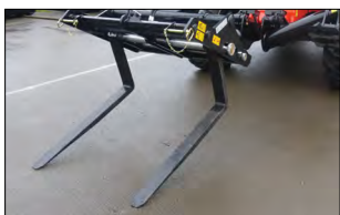
Floating forks with levelling
