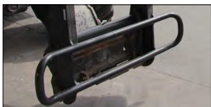
Anti-swing bag stabilizer- increases stability
