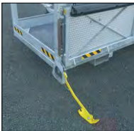
2 roof presence sensors
