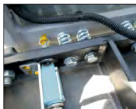
Overload, roof presence & physical locking sensor.
