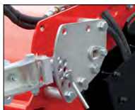
Interchangeable side brush (left or right)
