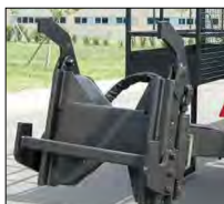
Hydraulic rib clamp- opening 325 - 482mm
