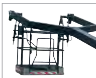
Pendular platform allows work under-bridges
