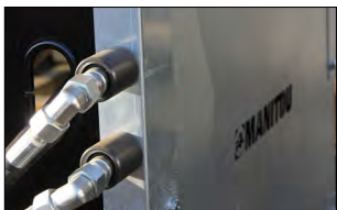
(1) Fully enclosed hydraulic components & connector sockets
