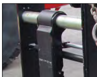
Fork positioning using sliders- forks keep floating
