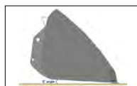
3° angle between the bucket's bottom line & the 500HB cutting edge for more longevity
