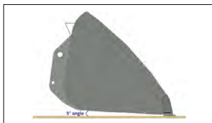
3° angle between the bucket's bottom line & the bolted cutting edge for more longevity
