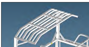
FOPS roof for a maximum protection
